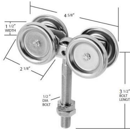
102-S1-T Vertically Adjustable Trolley Bolt is 1/2" x 3-1/2" with two hex nuts.
