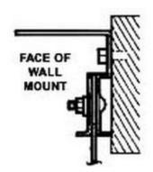
Face of Wall Mount PVC strips mount on the wall and hang over the door opening.
