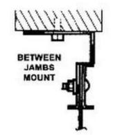
**Between Jamb Mount** PVC strips mount easily between door jambs.
