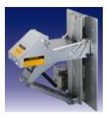
The ATL-450 Hydraulic Wall-Mounted Truck Restraint uses simple push button operation. It is easy to install and simple to operate. Vertical locking hook secures virtually all rear impact guards with excess of 32,000 lb. restraining force. It has a vertical operating range from 9" to 30".
