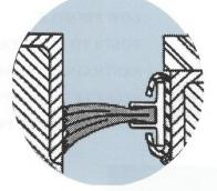
Seal Kit Includes: 2 Aluminum Side mtg. brackets 84" 2 Galvanized "C" Channels 84" 2 Nylon Side Brush Seals 1.5" x 84" 1 Foam Rear Seal 84"
