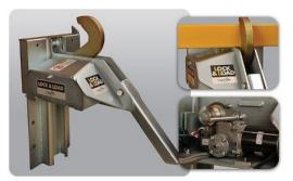
The Lock & Load is designed to secure a trailer to a loading dock by engaging the trailer's rear impact guard (RIG) with a large, rotating hook operated by a control panel mounted inside the building. Engagement range extends from 9" to 27" above the ground. A spring loaded, structural steel housing automatically positions the unit when contacted by a backing truck.
