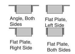
Bumpers may be ordered with angles or flat plates at each end. Use a flat plate for mounting bumper next to a dock leveler, or where the space is to tight to allow the use of angles. Note: When using the flat plate, it is welded to the dock.
