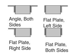
Bumpers may be ordered with angles or flat plates at each end. Use a flat plate for mounting bumper next to a dock leveler, or where the space is to tight to allow the use of angles. Note: When using the flat plate, it is welded to the dock.
