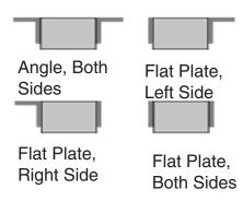
Bumpers may be ordered with angles or flat plates at each end. Use a flat plate for mounting bumper next to a dock leveler, or where the space is to tight to allow the use of angles. Note: When using the flat plate, it is welded to the dock.
